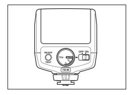
Sliding the power switch to the (ON) position will turn on the power. The ready lamp will light up when the flash is charged. Sliding it to the (OFF) position will turn off the power.
