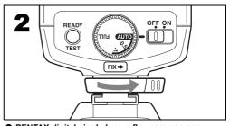
● PENTAX digital single lens reflex cameras can accept a shoe lock pin. When attaching the flash unit, turn the locking lever in the (FIX→) direction and lock the flash unit to the camera with the shoe lock pin. When releasing the flash unit, be sure to do so after turning the locking lever in the direction opposite to that indicated by (FIX→) and loosening the shoe lock pin. Otherwise, the hot shoe will be damaged.
