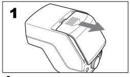
Slide the battery chamber cover as shown in the figure and remove it.
